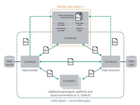
Figure 2 – A data platform in the Mobility Data Space extended by IDS components
