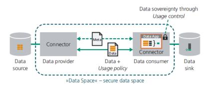
Figure 1 – Functional principle of data sovereignty through mechanisms for data usage control
